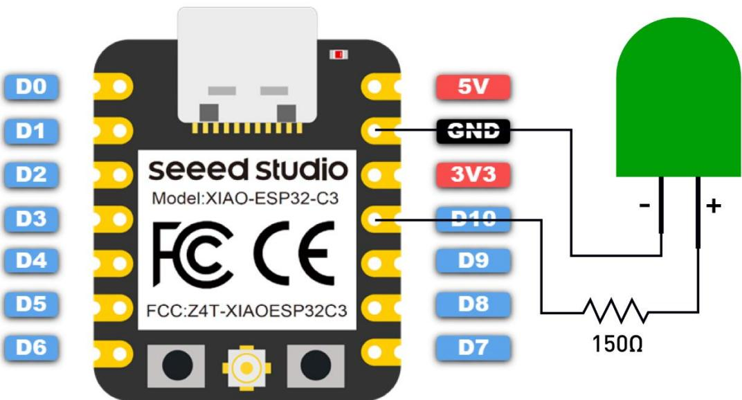
**Note:** Make sure to connect a resistor (about 150Ω) in series to limit the current through the LED and to prevent excess current that can burn out the LED
