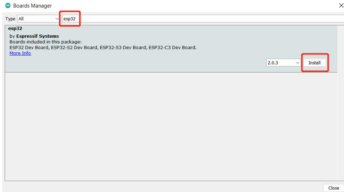
**Bonus steps - add XIAO ESP32C3 manually (This step will be changed after XIAO ESP32C3 shows up on Arduino Board Manager)**
