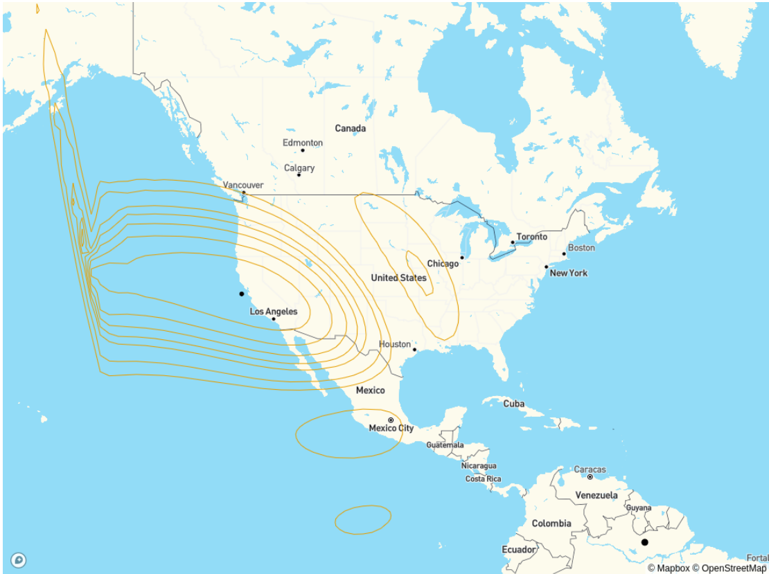
Figure A-1. Ku-band satellite transmit beam gain contours to be used during testing over the western United States
