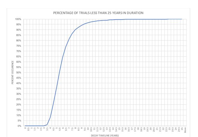
Figure 3: Monte Carlo Trials of Decay Timeline by Percentile (5000 trials)
