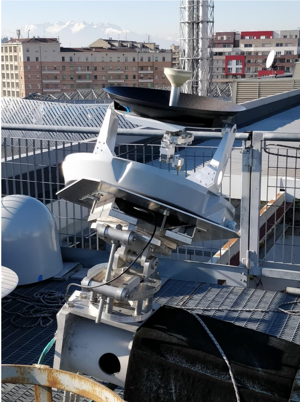
Fig.5: Antenna BBIG45Ku mounted on AUT positioner.
