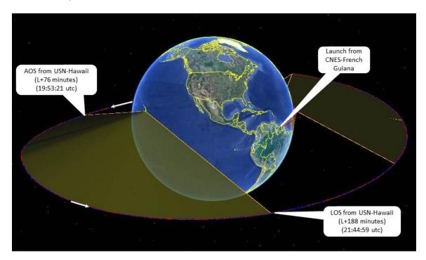
Figure 1 - O3B-VS10 Launch vehicle coverage from Hawaii
