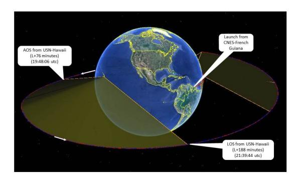
Figure 1 - O3B-VS06 Launch vehicle coverage from Hawaii
