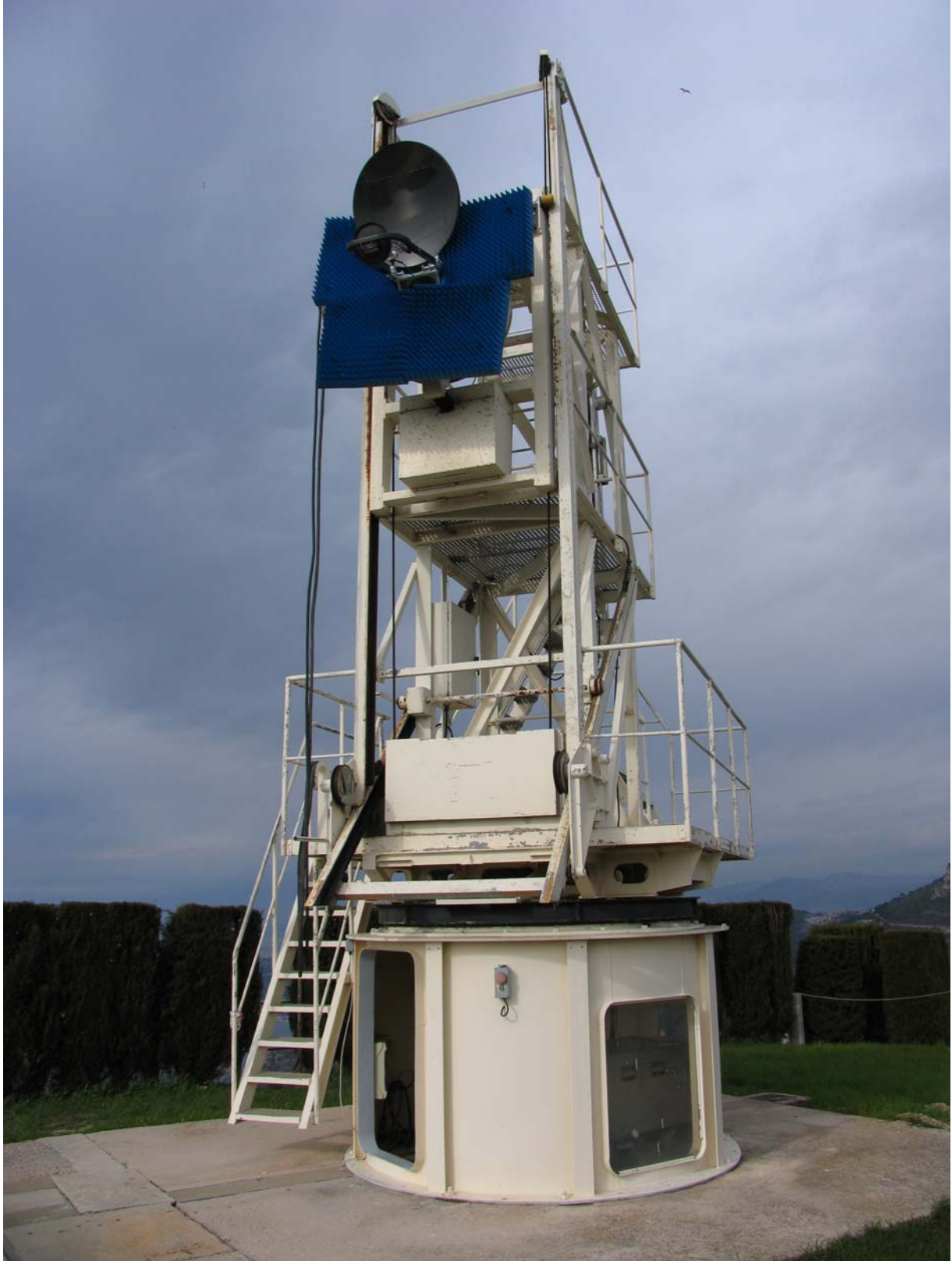
LightAway antenna on RF test bench (1/2)
