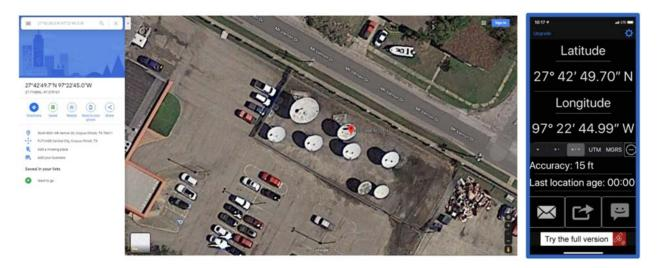
In light of the foregoing, the license coordinates for E050060 should be corrected to the GPS coordinates taken at the base of the antenna, which are within 3" of the licensed coordinates: 27° 42′ 49.7 N 97° 22′ 45.0 W (27.713806 N 97.379167 W).
