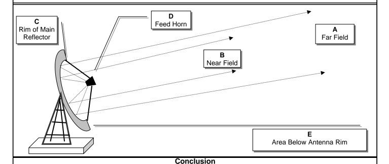
The results of this study indicate that accessible ground level areas, surrounding the antenna base and horizontal to the main beam axis, do not exceed the most restrictive FCC General Population/Uncontrolled MPE limit.
