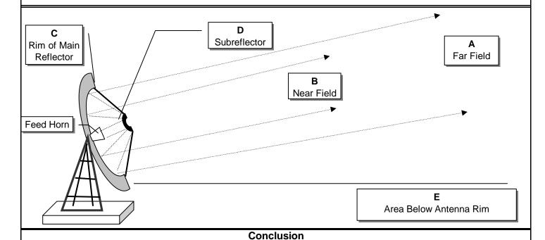
The results of this study indicate that accessible ground level areas, surrounding the antenna base and horizontal to the main beam axis, do not exceed the most restrictive FCC-General Population/Uncontrolled MPE limit.
