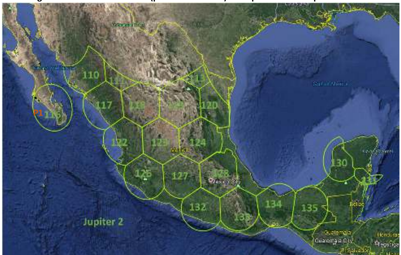
Figure 1: Thales ESAA Operating on AMC-15 – New Beam pointing Shows Worst Case Skew Angle of 40° and elevation 15° (position P1 in red) for repositioned Ka Spot Beams
