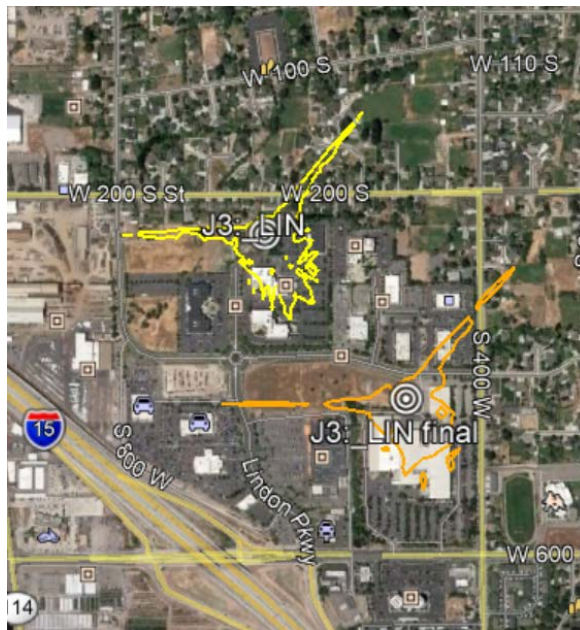
Figure 10. Section 25.136 pfd contours around the Lindon earth station in the 50 GHz band at the old site location (yellow) and the new (orange)
