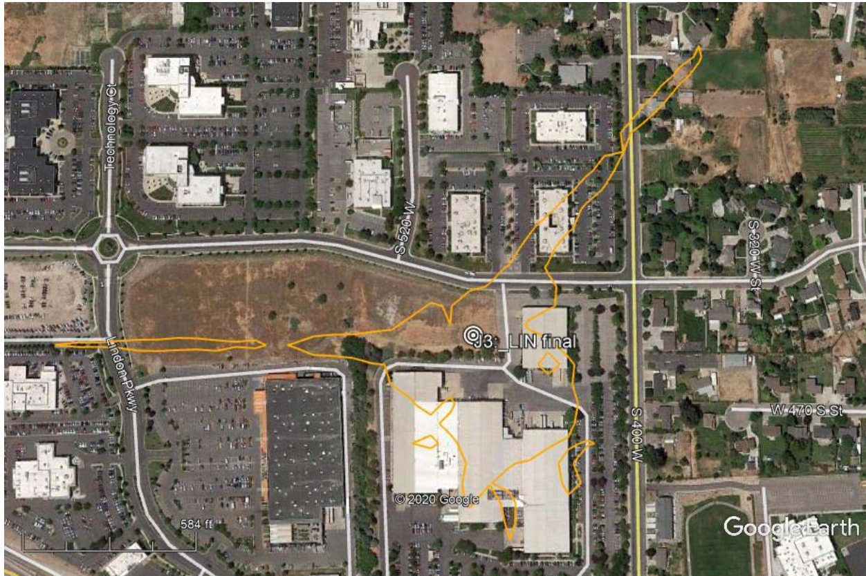
Figure 7. Section 25.136 pfd contour around the Lindon earth station in the 47 GHz band
