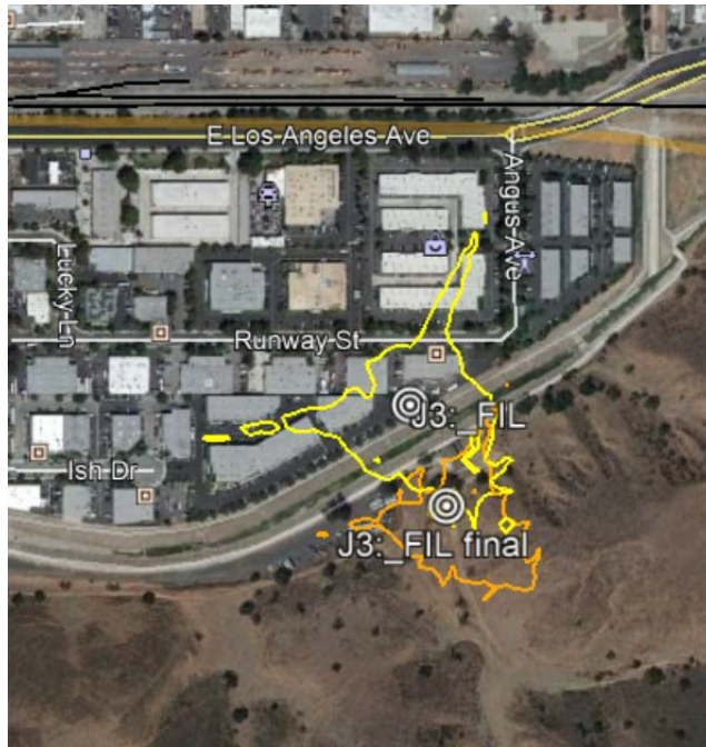
Figure 8. Section 25.136 pfd contours around the Simi Valley earth station in the 50.9 GHz band at the old site location (yellow) and the new (orange)
