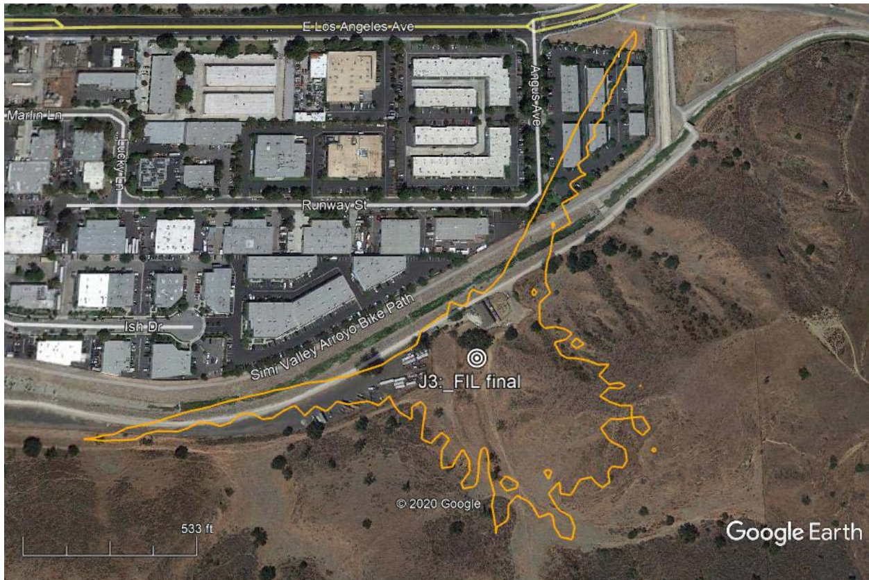
Figure 2. Section 25.136 pfd contour around the Simi Valley earth station in the 27.5-28.35 GHz band
