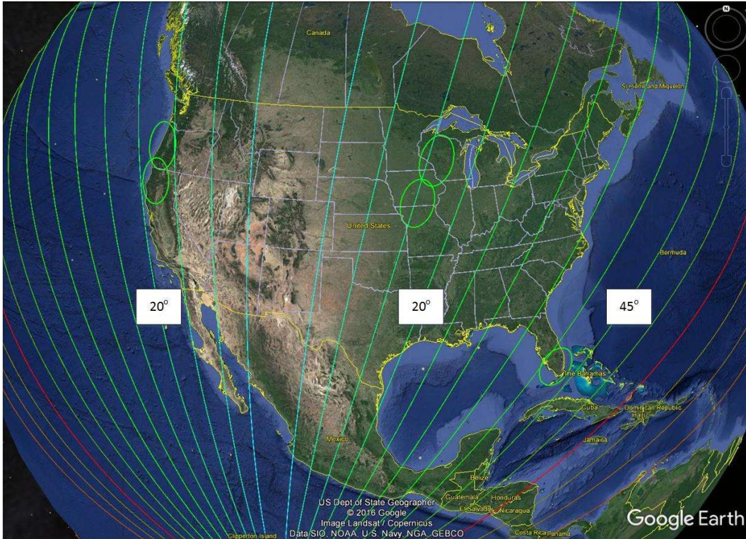
Figure 3: Thales's Jupiter-1 Coverage Area and Skew Angles (Worst-Case Skew 45°, Elevation 30°)
