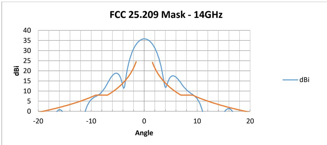
The symmetrical reflector's transmit pattern at 14 GHz is shown above overlaid with the 25.209 mask. Subtracting the mask from the pattern shows the excess gain:
