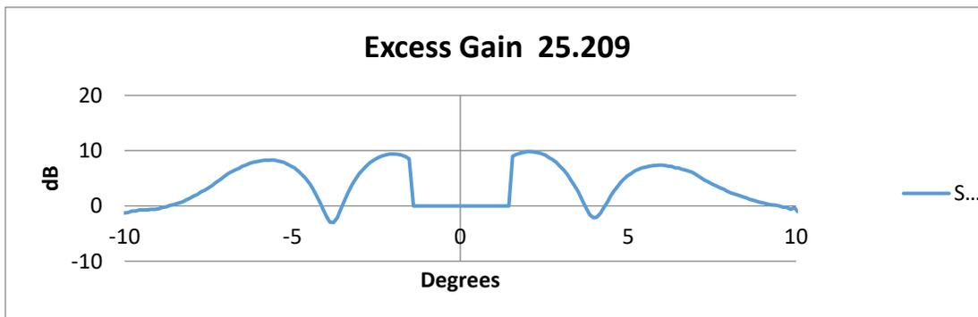
The small reflector cannot meet 25.209. It instead must gain compliance via lower power spectral density. These next plots show that if the antenna is limited to an ESD level of -23.5 dBW/4kHz at the feed input, it will be compliant with 25.226.
