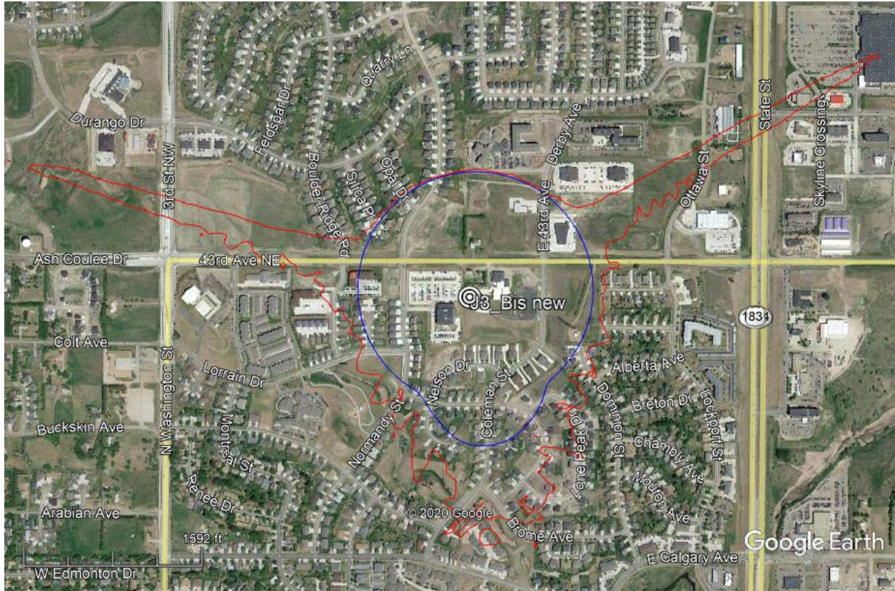
Figure 4. Section 25.136 grandfathered and aggregate PFD contours around the Bismarck earth station in the 27.85-28.35 GHz band
