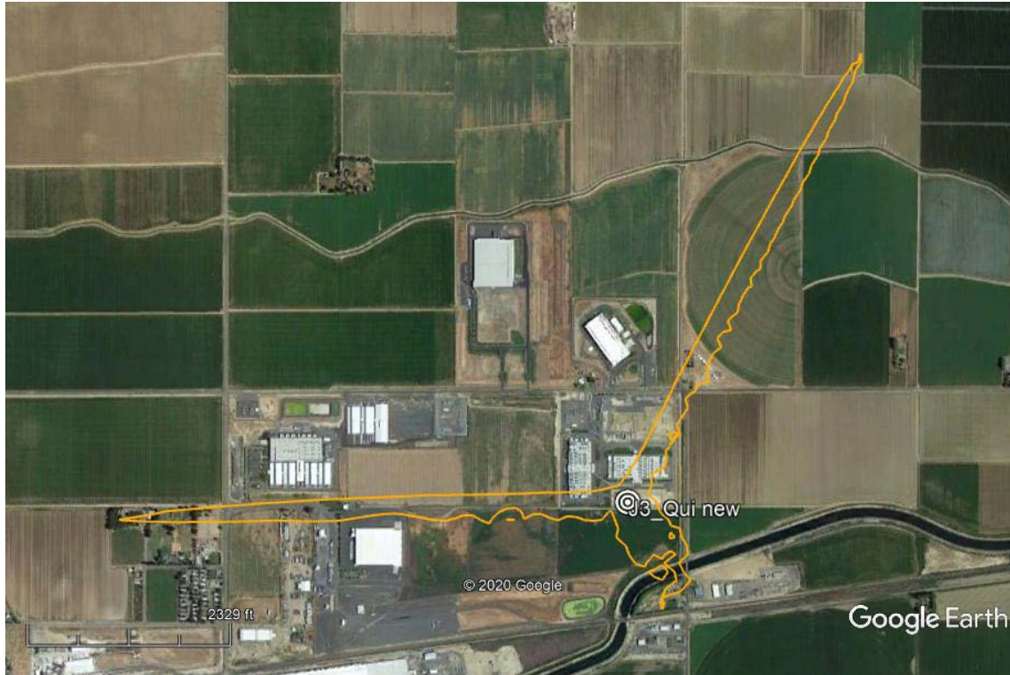
Figure 2. Section 25.136 pfd contour around the Quincy earth station in the 27.5-28.35 GHz band
