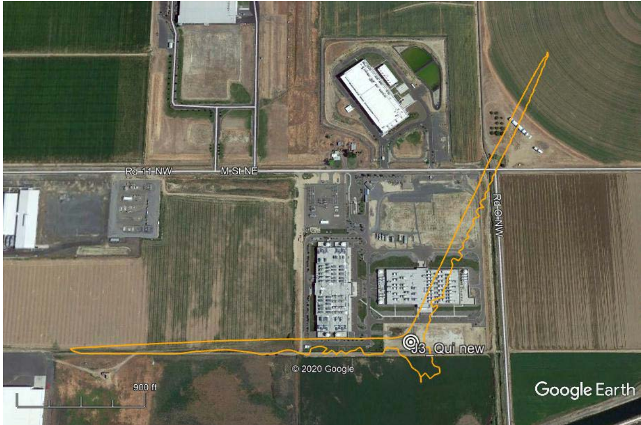
Figure 5. Section 25.136 pfd contour around the Quincy earth station in the 47 GHz band
