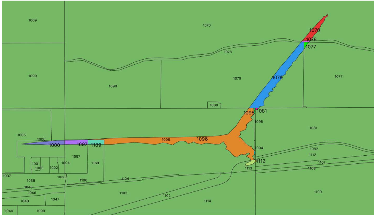
Figure 3. 27.5-27.85 GHz pfd contour overlaid on labeled census blocks
