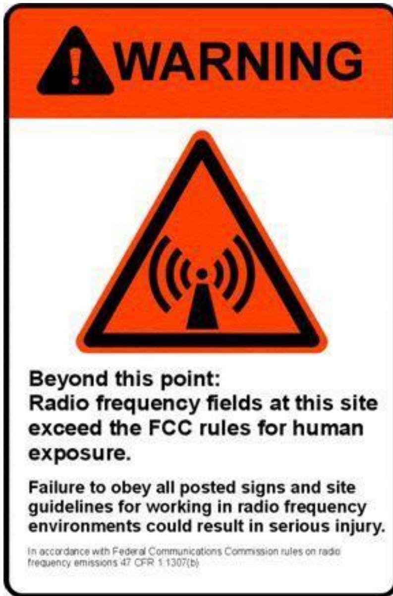
Figure 8 - Radiation Hazard Warning Label Sample
