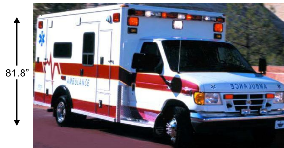
Figure 4 - Height at the Rooftop of an Ambulance (Type III)
