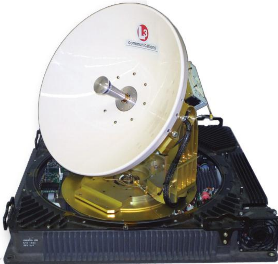
Figure 1. Photo of FSS-4180-LC with Radome Removed.
