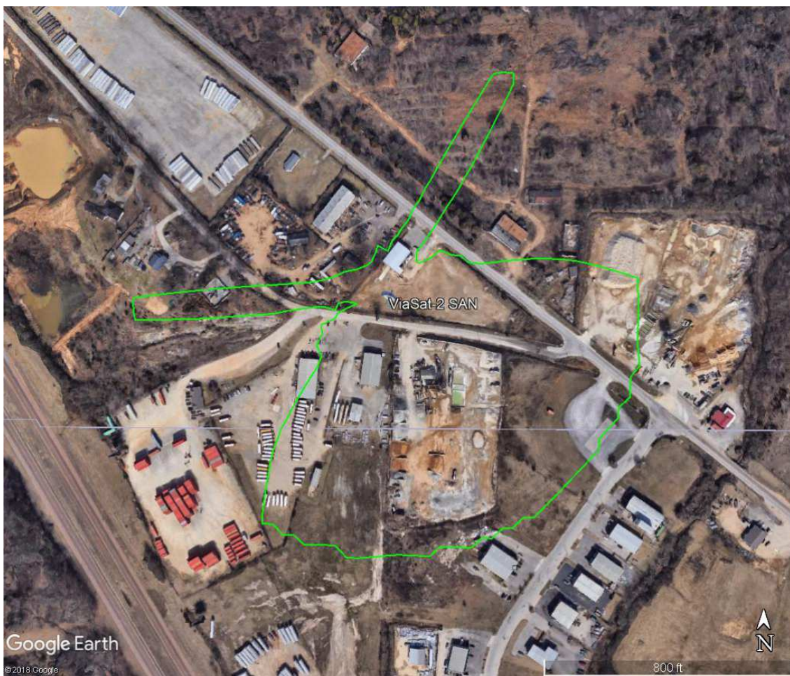
Area around proposed earth station location at Memphis, TN outside of which -77.6 dBm/m 2 per MHz threshold value measured at a 10-meter reference height is not exceeded
