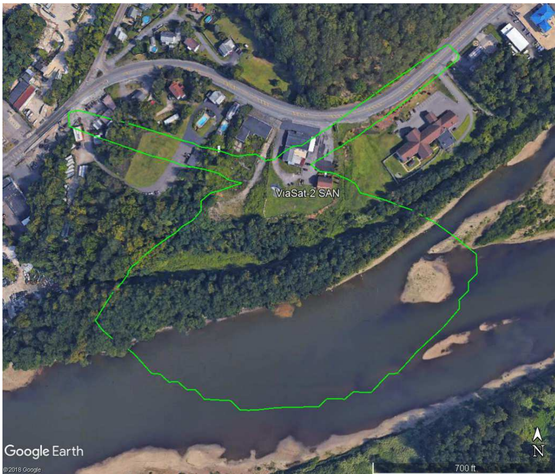
Area around proposed earth station location at Scranton, PA outside of which -77.6 dBm/m 2 per MHz threshold value measured at a 10-meter reference height is not exceeded
