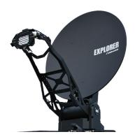
The required technical data for the 8100GX Earth stations is provided in the Form 312. In addition, for blanket licensing of transmitting Earth stations in the 29.5-30.0 GHz band, the Commission adopted off-axis EIRP spectral density levels contained in Section 25.138(a).
