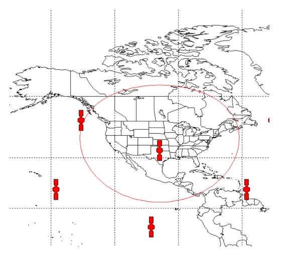
Representative 24-Satellite Constellation Footprint with user elevation mask at 5 degrees above the horizon:
