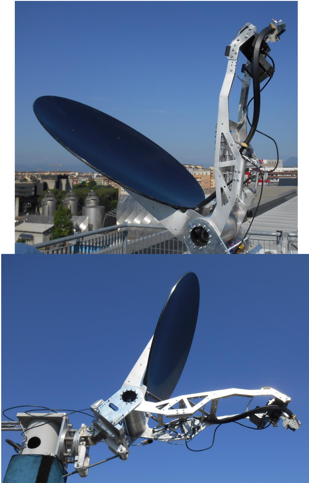
Fig. 7: The antenna mounted on the reclined and vertical mast.
