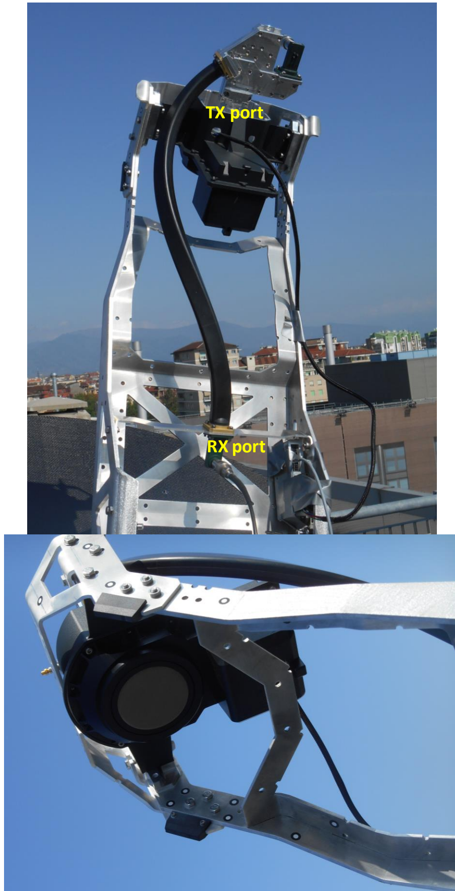
Fig.8: two views of the feed with the ports and the feeding flexguide.
