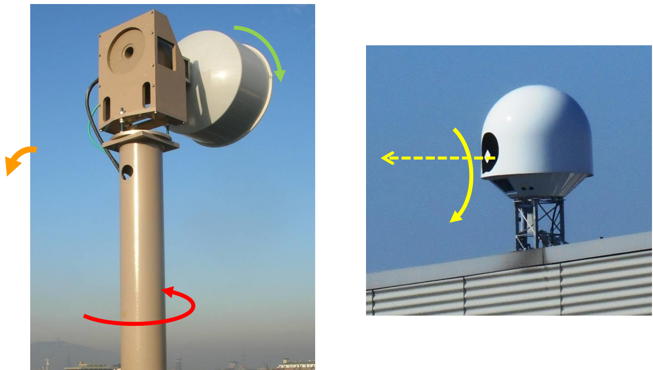
Fig.2: Outdoor test range: the AUT mount (left) and the upper SRC mount (right).
