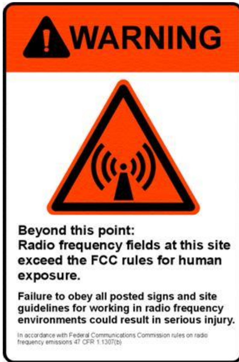
Figure 8 - Radiation Hazard Warning Label Sample
