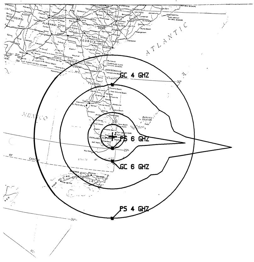
EARTH STATION NAME : MIAMI EARTH STATION STATE CODE : FL OWNER NAME : AMERICASKY LATITUDE : 25 48 35.0 North LONGITUDE : 80 21 11.0 West GROUND ELEVATION : 6.0 Feet AMSL CENTERLINE : 18.0 Feet AGL EASTERN ARC : 6.0 Degrees WESTERN ARC : 114.0 Degrees SATELLITE DEGREE SPACING : 1.0 Degrees
