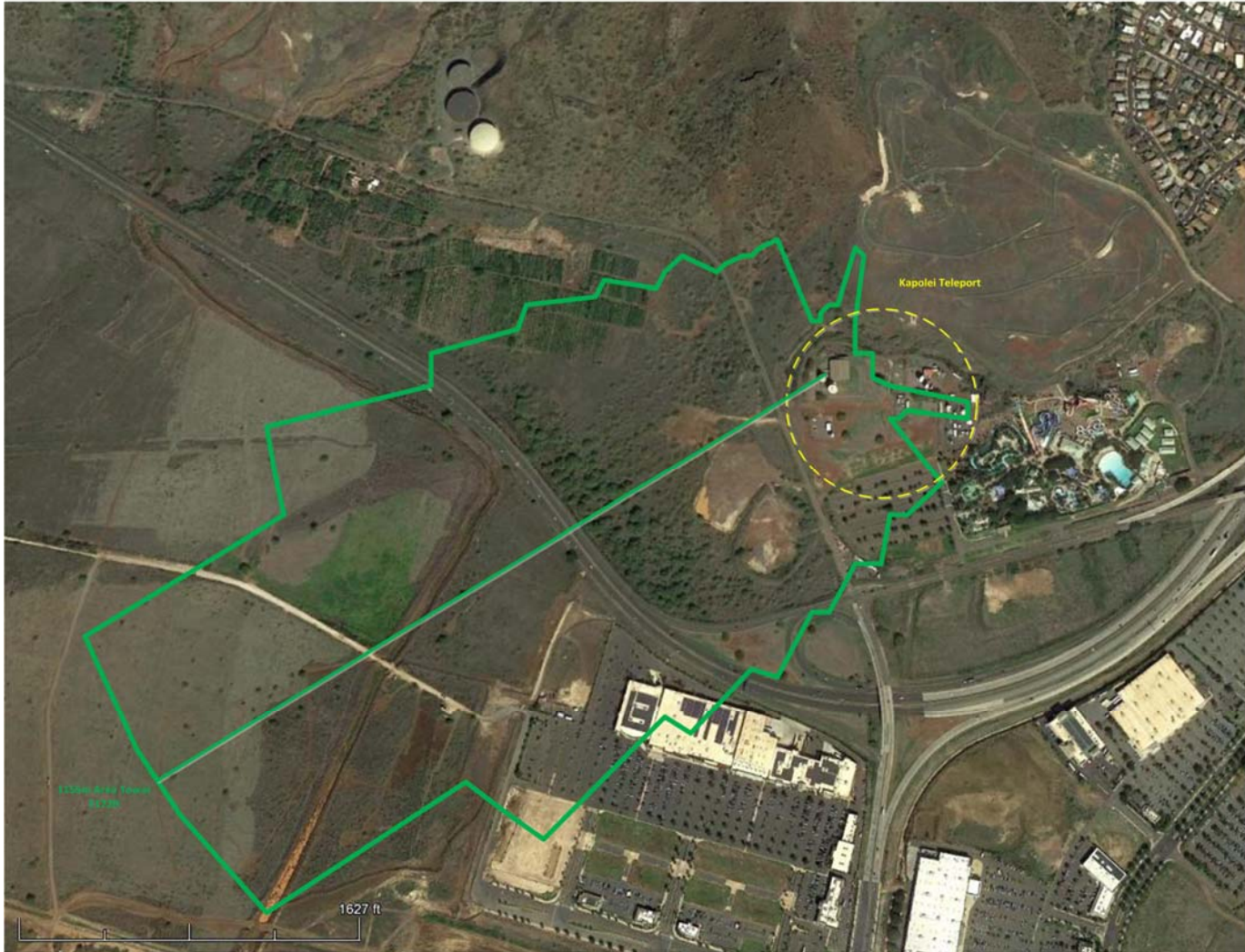
Figure 2 – HPT Kapolei Teleport: 25.136 -77.8 dBm/m 2 /MHz PFD Limit Zone
