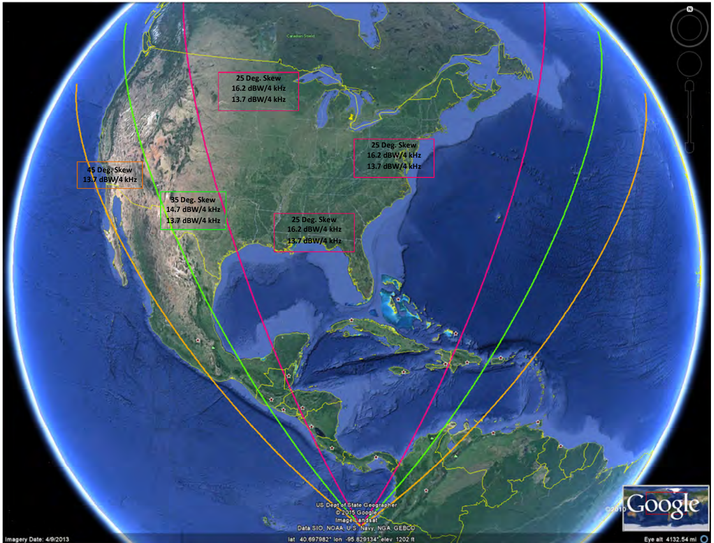
Figure C-27 Geographic skew boundaries and EIRP density levels for AMC-2 at 80.9 West. EIRP density limits are applicable anywhere between the associated left and right skew boundary contours. (Red: 25 degree boundaries; Green: 35 degree boundaries; Orange: 45 degree boundaries. Labels are located in the vicinity of areas of satellite coverage.)
