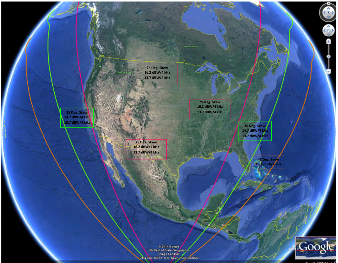
Figure C-25 Geographic skew boundaries and EIRP density levels for SES-1 at 101 West. EIRP density limits are applicable anywhere between the associated left and right skew boundary contours. (Red: 25 degree boundaries; Green: 35 degree boundaries; Orange: 45 degree boundaries. Labels are located in the vicinity of areas of satellite coverage.)
