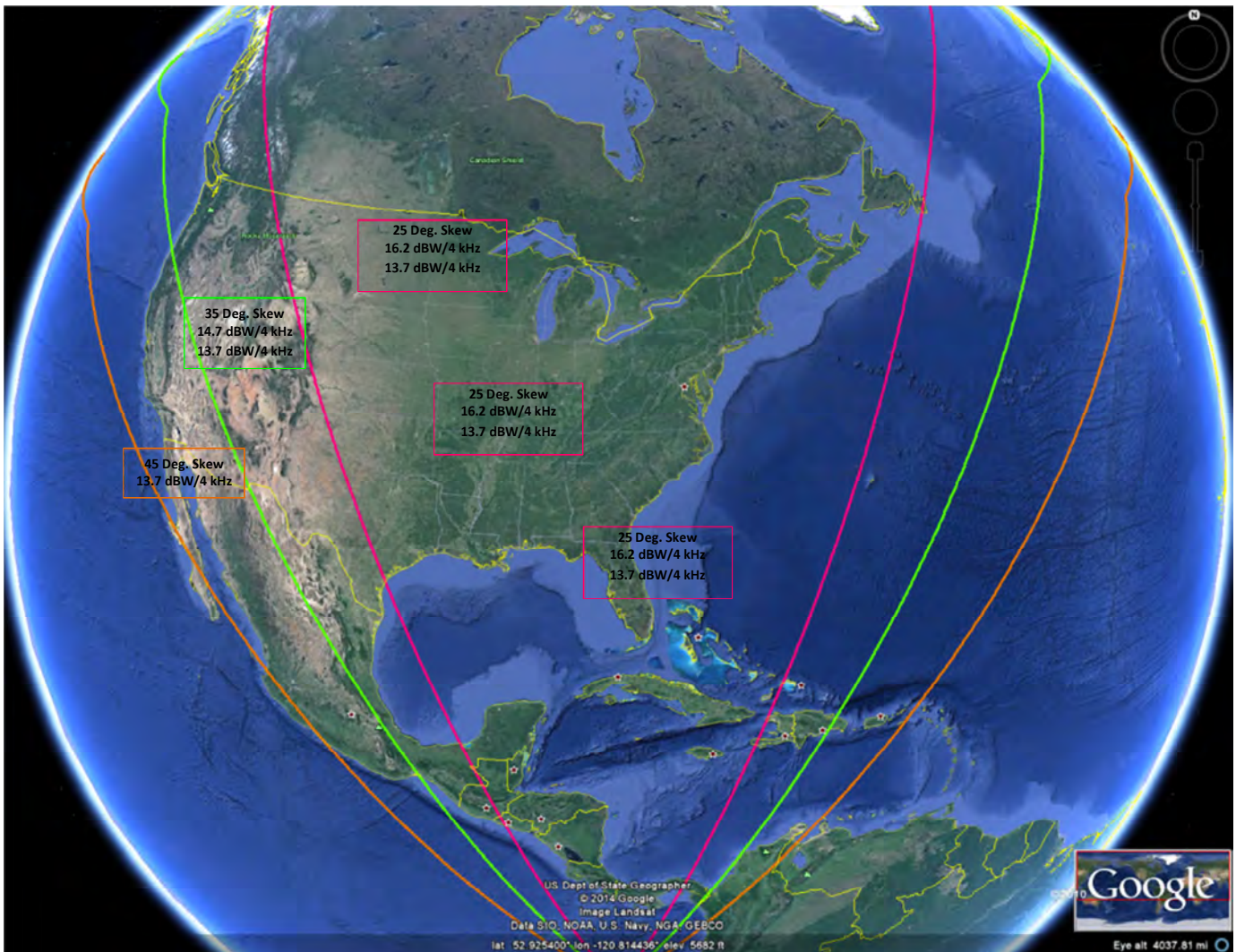
Figure C-26 Geographic skew boundaries and EIRP density levels for AMC-9 at 83 West. EIRP density limits are applicable anywhere between the associated left and right skew boundary contours. (Red: 25 degree boundaries; Green: 35 degree boundaries; Orange: 45 degree boundaries. Labels are located in the vicinity of areas of satellite coverage.)
