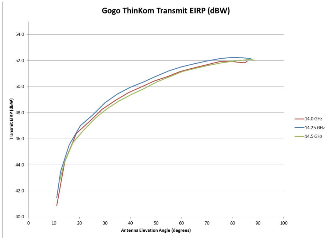
Figure 2 – Gogo ThinKom AES EIRP versus Elevation Angle
