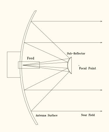
FIGURE 1. Satellite Antenna
