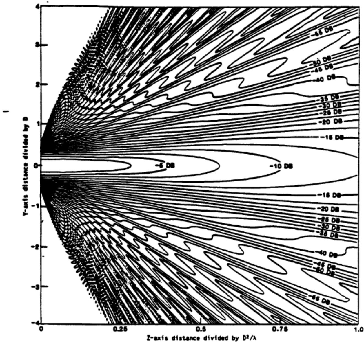
Figure 14. Relative Power Density Contours for a Circular Aperture Antenna. Contours are Shown in the  $y$ - $z$  Plane for the Case  $D \geq 30\lambda$ , where  $-4D \leq y \leq 4D$  and  $0 \leq z \leq D^2/\lambda$ . The Aperture Illumination is  $[1-(\rho/a)^2]^2$ , where  $\rho$  is the Radial Distance Variable,  $0 \leq \rho \leq a$ , and  $a = D/2$ . Each Contour Corresponds to an Increment of  $-2.5\text{dB}$ .
