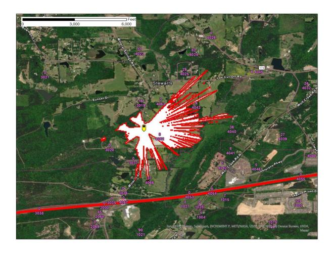
Figure 1 – Pell City, AL SAN -77.6 dB(mW/(m2 \* MHz)) pfd contour
