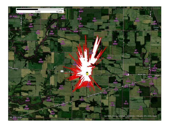
Figure 1 – Coatesville, IN SAN -77.6 dB(mW/(m2 \* MHz)) pfd contour
