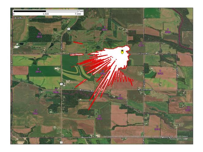
Figure 1 – Winslow, IL SAN -77.6 dB(mW/(m2 \* MHz)) pfd contour
