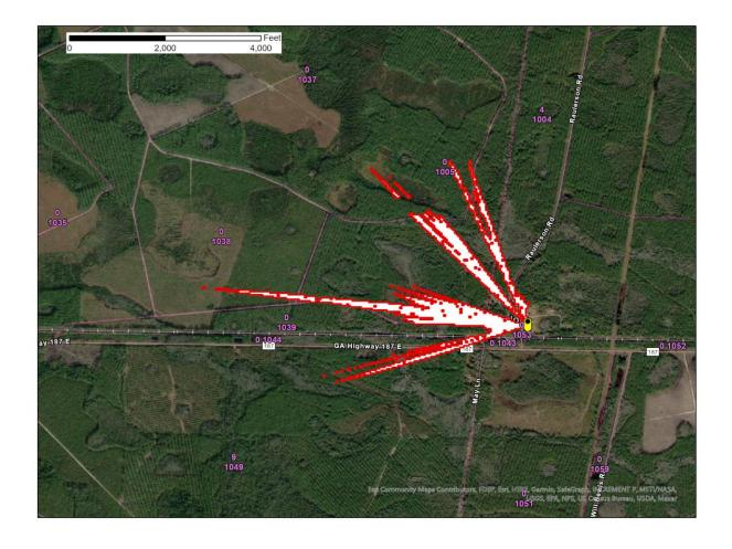
Figure 1 – Dupont, GA SAN -77.6 dB(mW/(m2 \* MHz)) pfd contour
