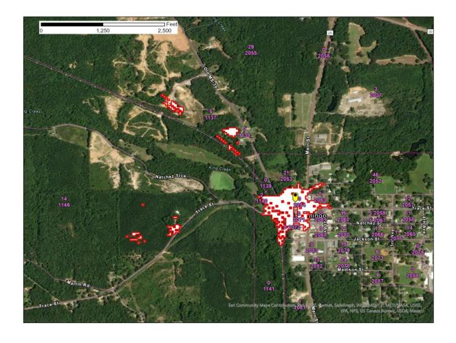
Figure 1 – Tishomingo, MS SAN -77.6 dB(mW/(m2 \* MHz)) pfd contour
