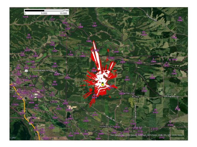
Figure 1 – Savanna, IL SAN -77.6 dB(mW/(m2 \* MHz)) pfd contour
