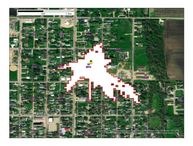
Figure 1 – Amboy, IL SAN -77.6 dB(mW/(m2 \* MHz)) pfd contour
