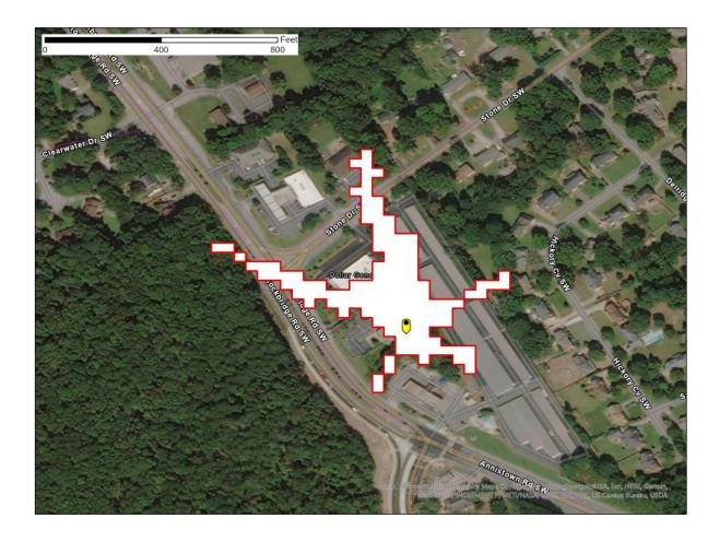
Figure 1 – Stone Mountain, GA SAN -77.6 dB(mW/(m2\*MHz)) pfd contour
