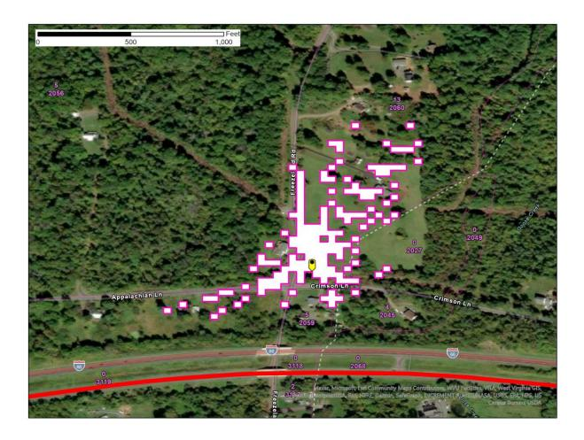
Figure 1 – Linden, VA SAN -77.6 dB(mW/(m2 \* MHz)) pfd contour
