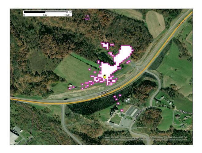
Figure 1 – Moorefield, WV SAN -77.6 dB(mW/(m2 \* MHz)) pfd contour
