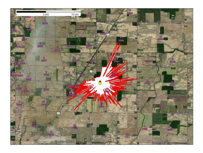
Figure 1 – Forest, OH SAN -77.6 dB(mW/(m2 \* MHz)) pfd contour
