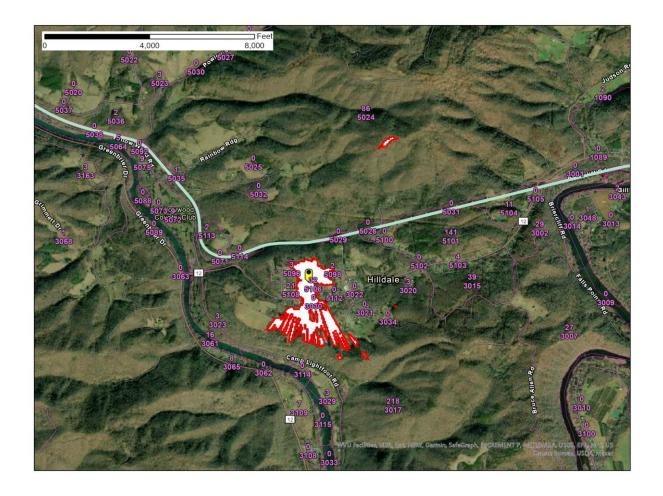
Figure 1 – Green Brier River, WV SAN -77.6 dB(mW/(m2 \* MHz)) pfd contour
