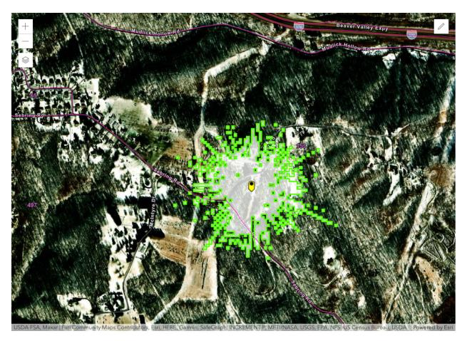
Figure 1 – Beaver, PA SAN -77.6 dB(mW/(m<sup>2</sup> \* MHz)) pfd contour
