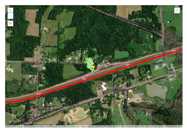
Figure 1 – Zanesville, OH SAN -77.6 dB(mW/(m<sup>2</sup> \* MHz)) pfd contour
