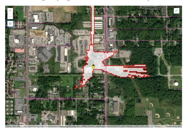
Figure 1 – Boardman, OH SAN -77.6 dB(mW/(m<sup>2</sup> \* MHz)) pfd contour
