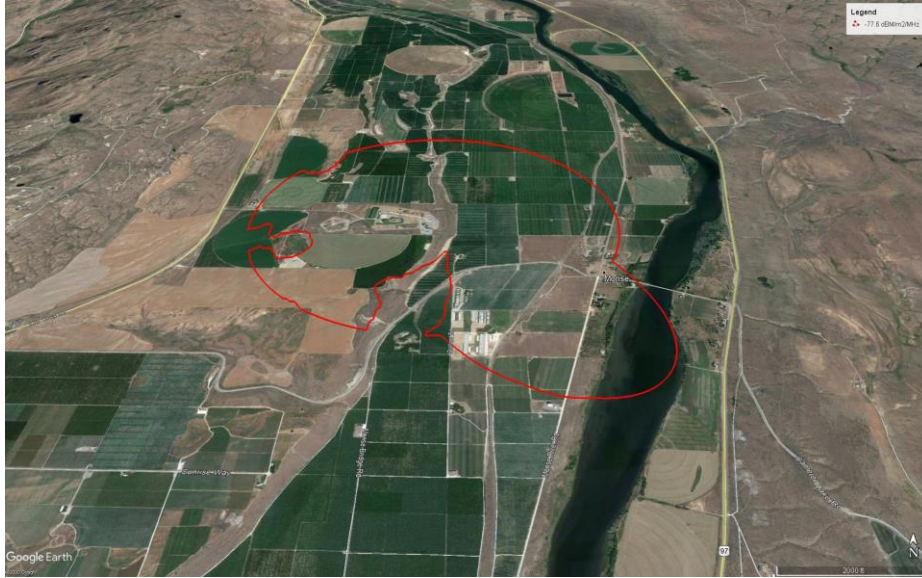
Figure 4. Case 2 projected PFD contour projected on an aerial image of the proposed location.
