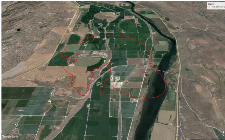
Figure 3. Case 1 PFD contour projected on an aerial image 8 of the proposed location.
