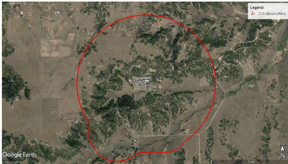
Figure 3. Case 1 PFD contour projected on an aerial image 8 of the proposed location.
