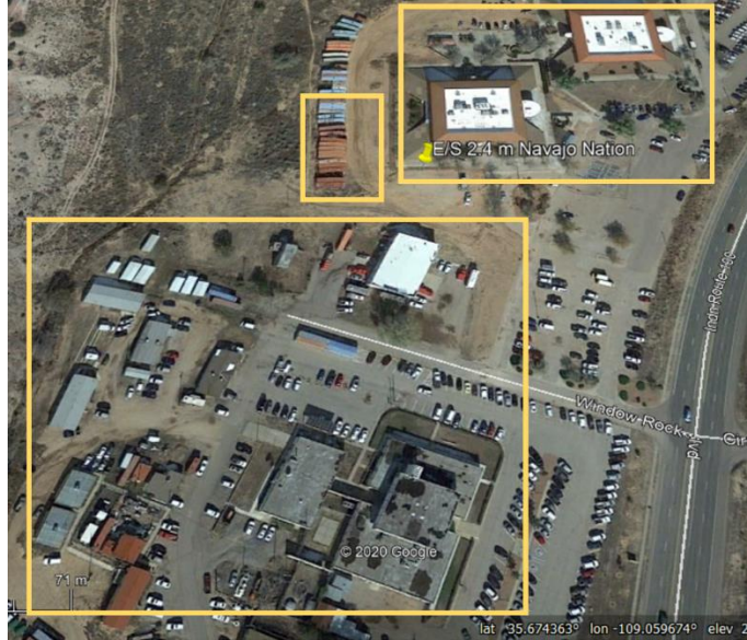
Figure 2: Picture of obstacles surrounding the antenna that were considered in the clutter analysis
