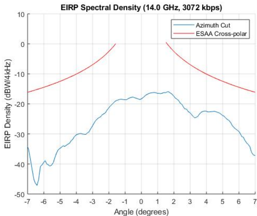
Figure 3-5 Cross-polarized Off-Axis EIRP Density in the plane of GSO Arc (14.0 GHz)
