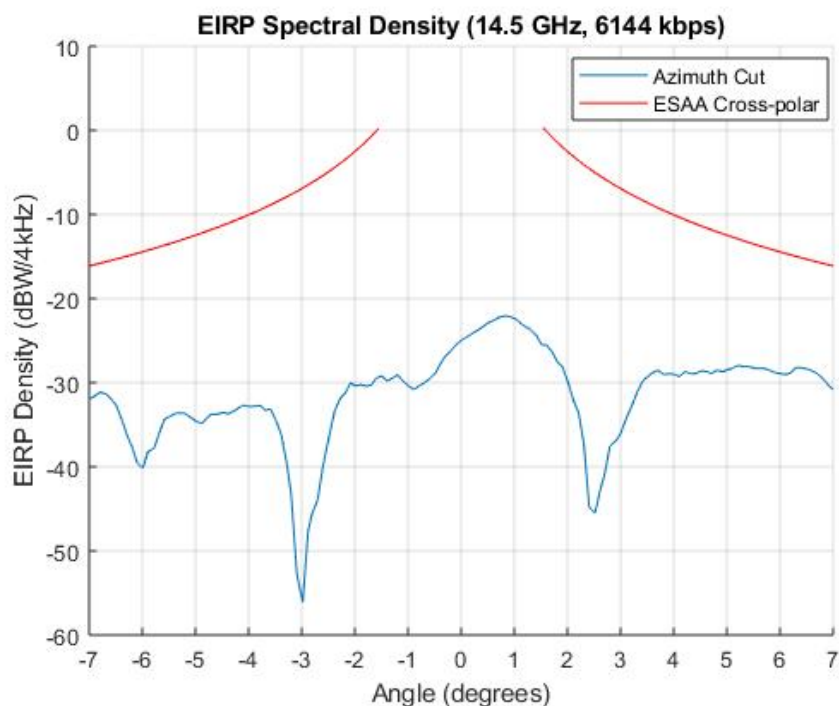
Figure 3-14 Cross-polarized Off-Axis EIRP Density in the plane of GSO Arc (14.5 GHz)
