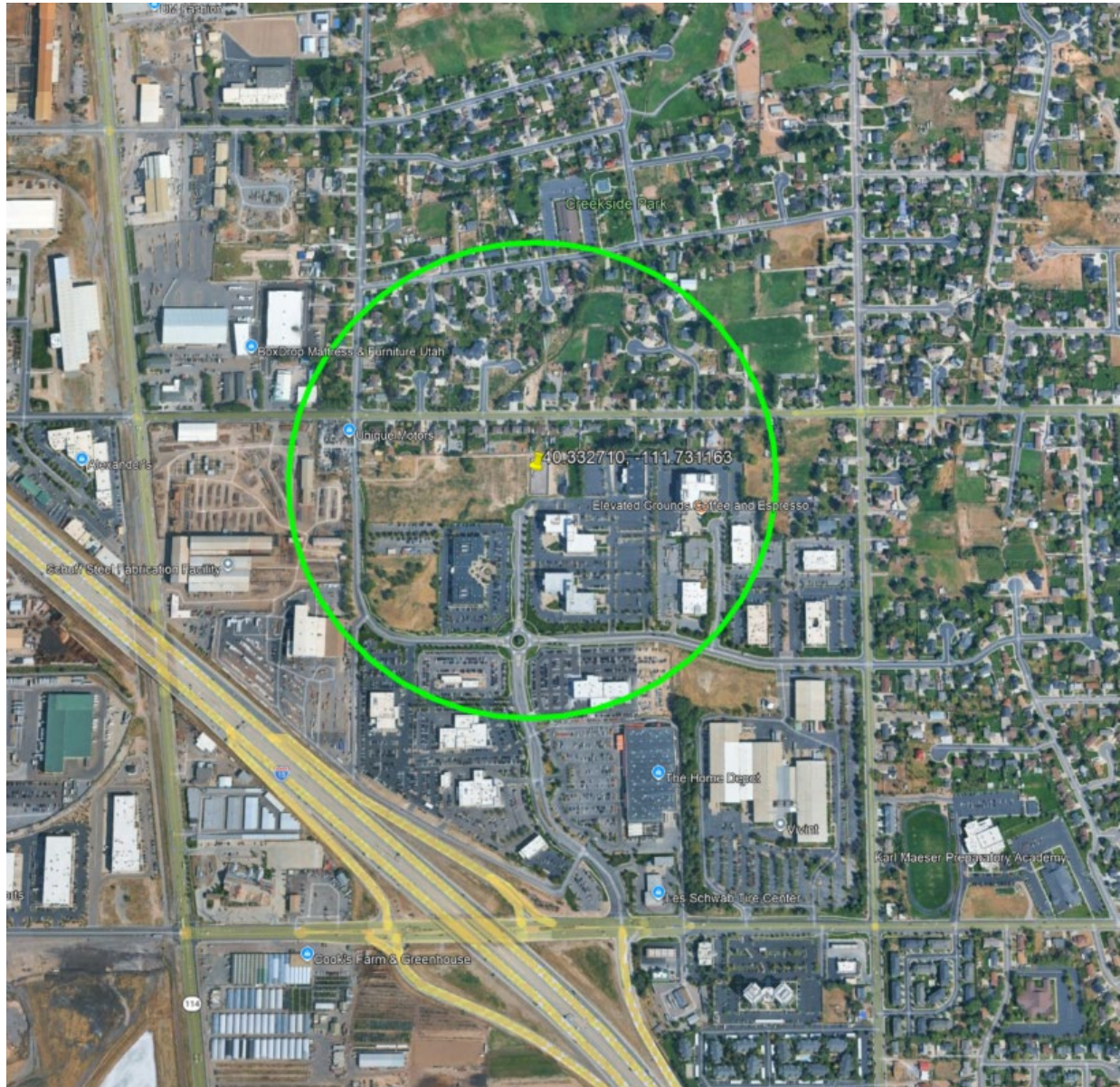
Figure 1. PFD Contour for the Gateway: V-band Uplink
